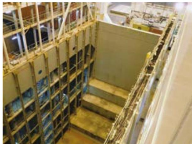
Figure 3: Typical containership cargo hold showing cell guides, source Captain Colin Fardy.
