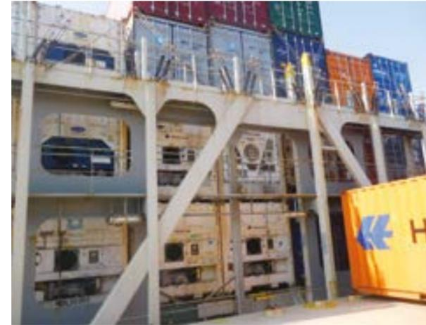
Figure 5: Refrigerated and standard containers stowed on deck, source Captain Colin Fardy.
