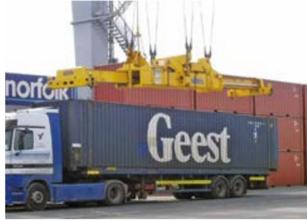
Figure 1: Container being lifted off a truck to be loaded on the ship, source Captain Peter Walter.
